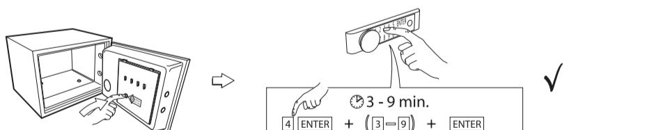
**!** If the wrong code is entered more than 5 times the safe will lock down for a period of time that can be set to 3-9 minutes.
