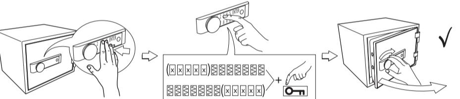
**!** A scramble number input enables personal codes to be hidden within longer sequences of numbers. The scramble number can be used either before or after the user code.
