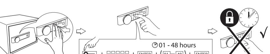
**!** To prevent any access to the safe you can manually lock the safe down for 01-48 hours.
