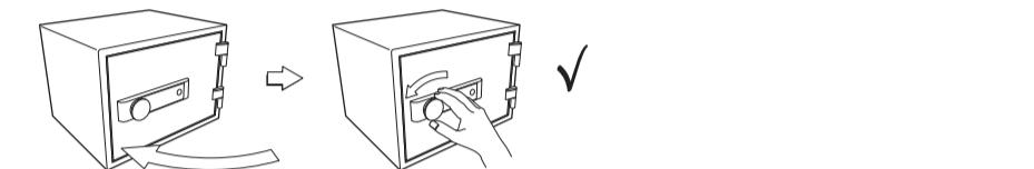
**!** When closing the door ensure the bolts are fully retracted and that the knob can't be turned to the open position.
