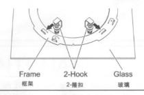
Make sure to tighten the four screws so that the packing between the frame and the glass is flattened. psg4個螺絲以確保框架與玻璃間的墊料被壓扁。
