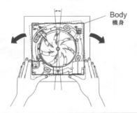
9 Secure the body and the frame with four screws after confirming the position.
