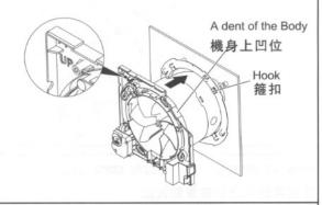
Rotate the body to adjust the horizontal and the vertical. Insert the body completely until the back of the body touches the glass.
