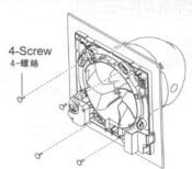
10 Secure the cover with three screws, be sure not to crimp any wires with cover. Hang the louver on the projections of the cover and press the louver at the lower side to fit into the cover.
