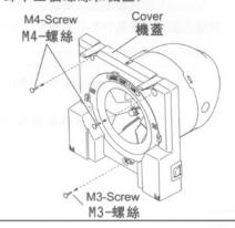
7 The UP mark of the body come to the up position. Aline a dent of the body to the hook of the frame, then insert the body to the frame carefully. 使機身上的 "up" 標志朝上。必須調整機身上的凹位使之對准框架上的箍扣,然後將機身小心地插入框架中。
