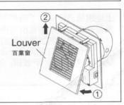
2 Turn the orifice counterclockwise. remove the orifice.
